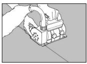
The sheets are hot welded. Do not weld until the adhesive has bonded completely, wait 24-48h. The joints are chamfered or grooved to about 3/4 of the thickness using a hand grooving tool or machine prior to welding.
