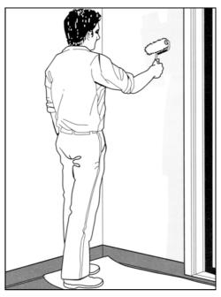
Apply adhesive on the wall area where the first sheet will be installed and a few inches past the seam edge. Apply adhesive in accordance with manufacturer's instructions. Use a 'lambs hair' roller. If you prefer to apply the adhesive with a fine-notched trowel, we recommend that you even out the adhesive over the surface with a roller-otherwise there is a risk that the trowel pattern in the adhesive will later show through the wall covering.
