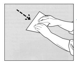
Press the sheet firmly using a piece of board with rounded edge or equivalent tool. Work from top down and from the middle to the sides of the sheet. **IMPORTANT: Make sure you remove all trapped air.**
