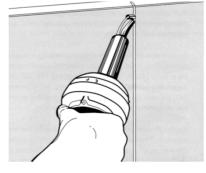
¬ Do not heat weld until the adhesive is completely dry, normally one day after installation.
