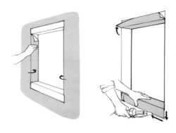
For best result, extra heating and pressing is necessary to secure a good bonding at overlapping areas.
