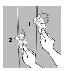
→ Welded seams must be allowed to cool to room temperature before they are trimmed. For best results, trim excess welding rod in two stages.
