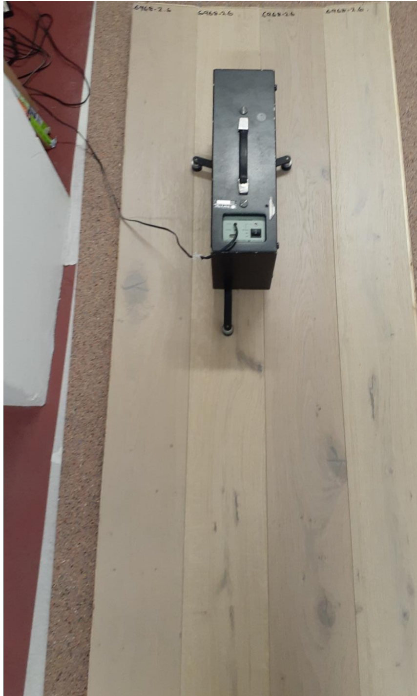
Figure 3 - WOOD 14/3mm CN Construction (OAK) with 2 mm Damtec colour underlay on base floor
