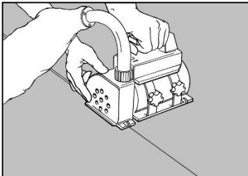
The sheets are hot welded. Do not weld until the adhesive has bonded completely, wait 24-48h. The joints are chamfered or grooved to about  $\frac{1}{4}$  of the thickness using a hand grooving tool or machine prior to welding.
