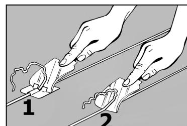
**CAUTION:** Welded seams must cool to room temperature before trimming. Start trimming where you began welding. All trimming of welding thread is recommended in two steps: rough and fine trimming.
