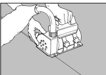
The sheets are hot welded. Do not weld until the adhesive has bonded completely, wait 24-48h. The joints are chamfered or grooved to about  $\frac{3}{8}$  of the thickness using a hand grooving tool or machine prior to welding.
