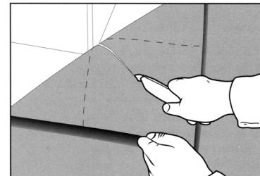
When fitting an out-corner, the sheet is folded against the corner and cut about 5 mm(  $\frac{1}{4}$  in.) from the floor. The guidelines in the picture show the corner on the sheet and the position of the cut at about a 45-degree angle. Then a diagonal cut is made as shown.
