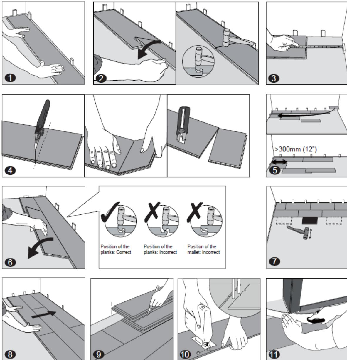
1. First row, first plank: After thoroughly cleaning the subfloor, you should begin laying from left to right. Position the first plank so that the grooved edge is facing you. Place the floorboard 6mm from the left wall. Use spacers between the wall and the floorboard.
